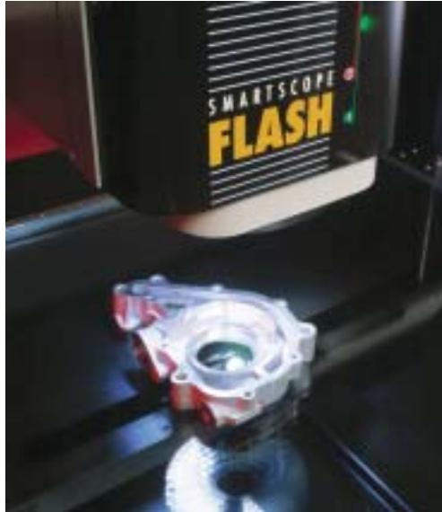
A video measurement of a cast metal part is illuminated by an LED ringlight.
