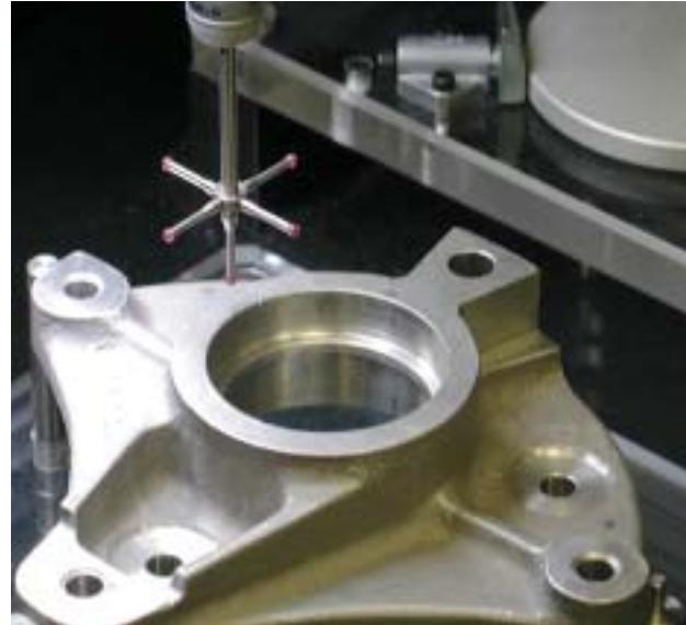
A star touch probe measures a cast metal part on a multisensor measurement machine.
