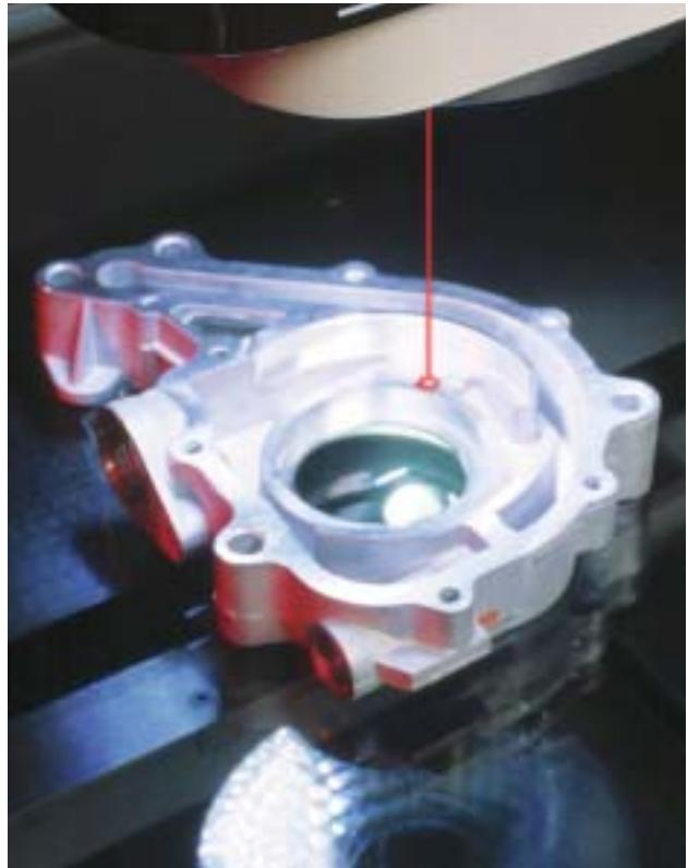
Through-the-lens (TTL) laser measurement of a surface.
