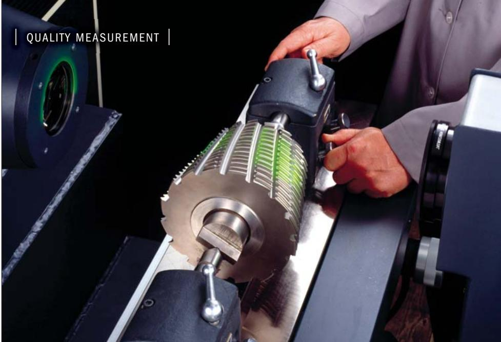
Random flaws and indistinct, variable features are difficult to program on an automatic video system, but can be easily accomplished with a contour projector. Source: Optical Gaging Products Inc.
