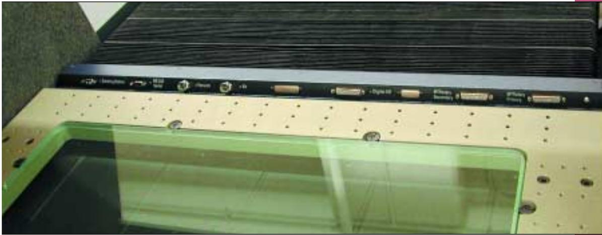
For part-fixturing needs, the Quest 650 sports a prewired panel featuring digital I/O ports for programmable fixturing, RS232 communication ports, air and vacuum ports, and other options.
