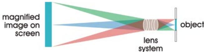
All comparators magnify an image and project it against a glass or plastic screen, which is viewed by the operator. In this case, the viewing screen performs the same function as the eyepiece lens of a microscope. The magnification of the lens system and the diameter of the viewing screen determine the field of view and associated resolution. *Source: Optical Gaging Products Inc.*
