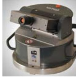
The LaserTRACER's core component is a laser interferometer that automatically follows a reflector and continuously measures the distance to it.
