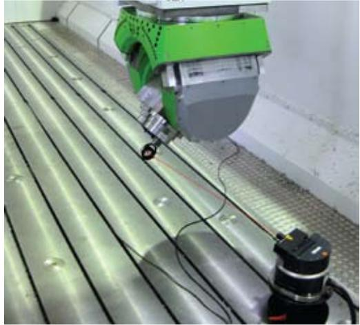
Determining the volumetric accuracy of large machine tools such as this portal mill is becoming a maintenance priority. In this application, the reflector is mounted in the spindle in place of a cutting tool.
