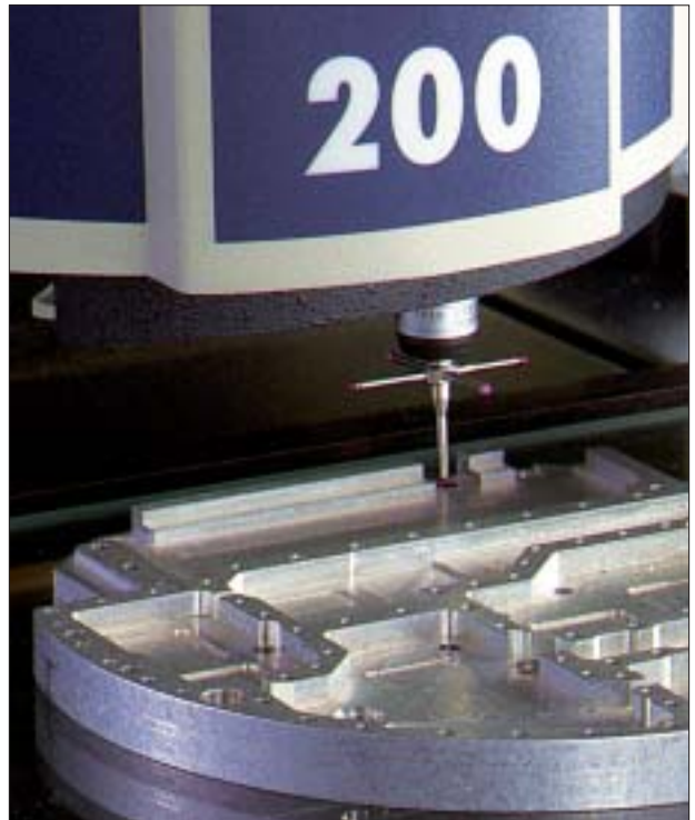
A star touch-trigger probe is used on a video-based multisensor measurement system. Source: Optical Gaging Products Inc.
