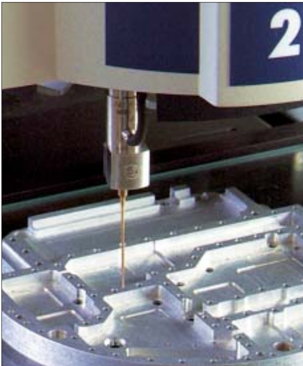
A microprobe is used on a video-based multisensor measurement system. Source: Optical Gaging Products Inc.
