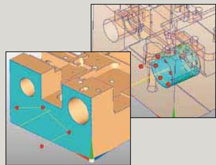
Assume the blue-highlighted edges in the CAD model in Figure 2b need to be measured to determine the relationship (distances) between them. Either of those edges can be assumed to be the intersection where perpendicular surfaces meet.
