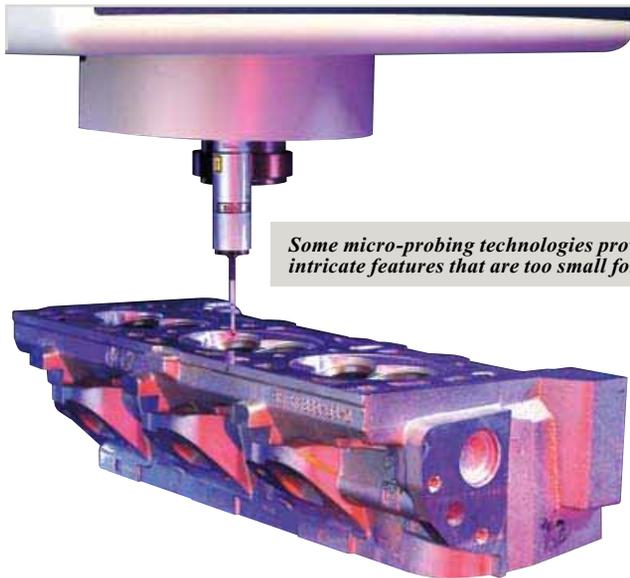
*Some micro-probing technologies provide access to intricate features that are too small for touch trigger probes.*
