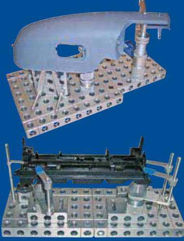
Alufix is a modular, highly accurate and reusable workholding system made of high-tensile Aerospace Aluminium. It is used for assembling all kinds of measuring fixtures, checking gauges, assembly fixtures, cubings, basic frames etc.
