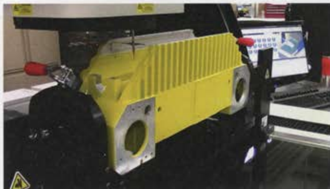
Fig. 3. Multisensor measurement of a large machined casting. Source: QVI
