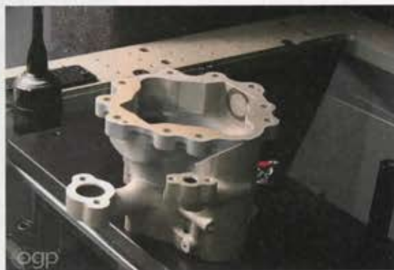
Fig. 4 Long working distance sensors are used to measure this housing. Source: QVI
