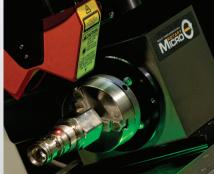
Laser and white light sensors excel at measuring complex curved surfaces and profiles.
